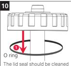
The lid seal should be cleaned and checked for wear when servicing *MagnaClean*. It is Best Practice to replace the lid seal at each service.
