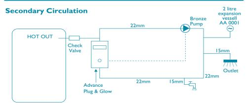
Set the Advance Plug & Glow at 45°C to maintain temperature in the secondary loop without affecting the store temperature, costing just pennies per day.
