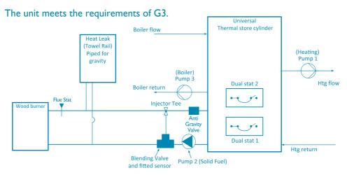
This schematic is for solid fuel pumped circulation.
