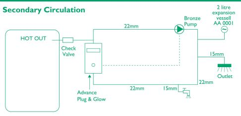
Set the Advance Plug & Glow at 45°C to maintain temperature in the secondary loop without affecting the store temperature, costing just pennies per day.
