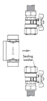
Slip the connector block between the isolation valves, taking particular care to ensure that the directional arrow on the connector block is pointing in the direction of the flow of water. Failure to do so will result in reduced flow and inhibited filter performance.
