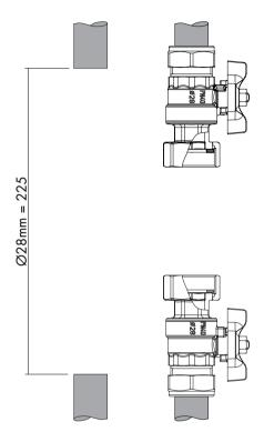
Having removed the prescribed section of pipework (as above), make sure that the open ends of both pieces of pipework are free of debris and ready to receive the nut and olive. Fit both isolation valves but do not tighten fully.
